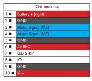
105 pads for Motor 7/8 and LED STRIP, 10 and accessory power.
