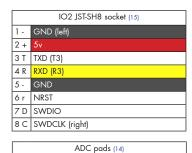
101 socket for UART3 and SWD debugging (Only fitted on NANO-E)
