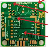
FC UART 4 = Stacking VTX UART1 - configure UART4 for RX and use the UART1 pads for the FrSky XM+ or Crossfire NANO RX.
